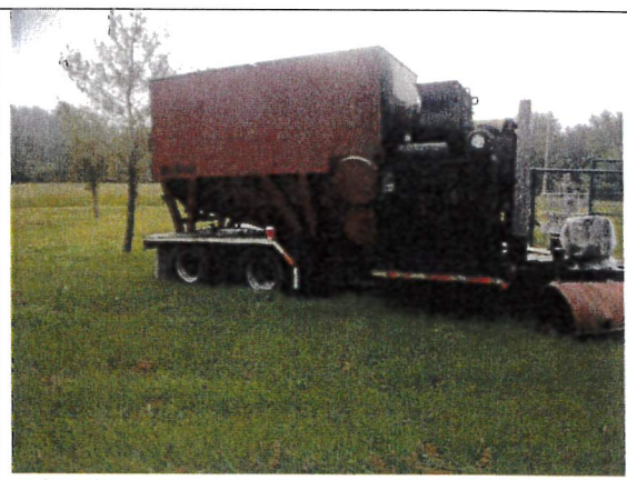
Dust collector on site.
